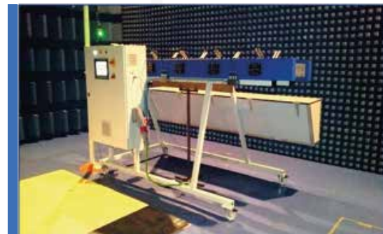
Fig 3. Heating and Vacuum System during EMC tests
