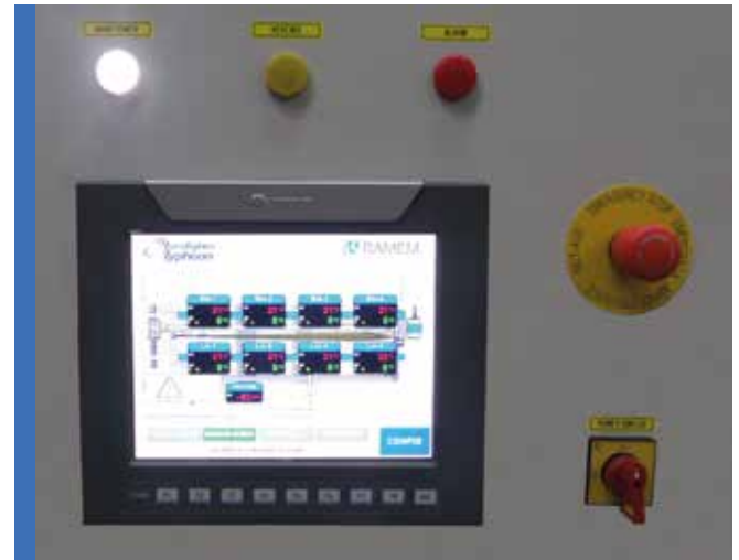
Fig 4. Heat controlled in 8 areas
